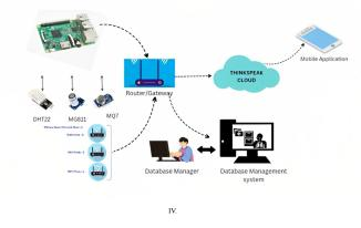
Fig. 1. Basic Architecture of Proposed System
